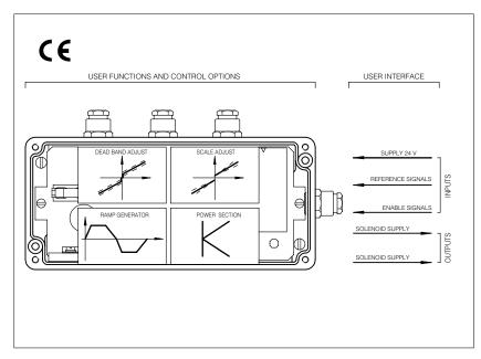
1 MODEL CODE E-RP AC 01F E-RP = Electronic Set code (see 4.4) driver Series number = 24 Vpc power supply = 12 Vpc power supply (see 4.1) AC = for proportional valves without transducer Options = standard symmetrical ramp /RR = with adjustable dissymmetrical ramps /RRE = with external ramp setting **01F** = for single solenoid proportional valves **05F** = for double solenoid proportional valves = suitable to receive current reference signal 4 ÷ 20 mA
